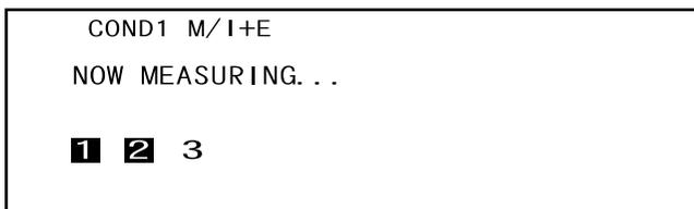
When the specified number of measurements has been completed, the averaging result will be displayed on the LCD.
