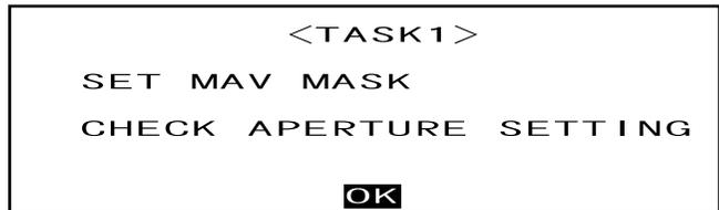
**6** Check the Target Mask and measurement area selector switch, then press
